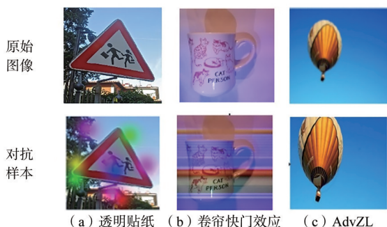
图10 针对摄像机的物理域对抗攻击 Figure 10 Physical-domain adversarial attacks against the camera
